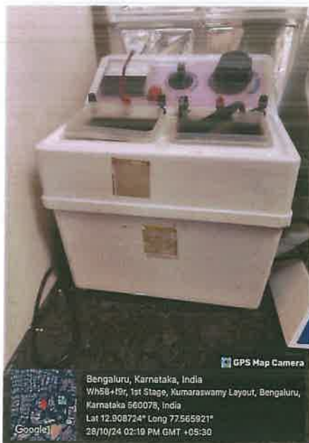
Electro polisher - to polish metal casting electrolytically
